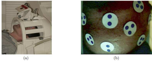
Fig. 1. [(a)] MR compatible cameras attached to the camera holder, which is attached to the MRI head coil. [(b)] Image of a volunteer as seen by one of the in-bore tracking cameras. Blue dots on paper stickers are used for tracking.
